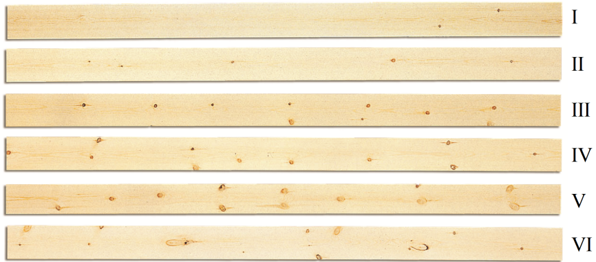
Figure 1.3: Example images of six standard NTGR grades of dimensions 50 \times 150 mm. From www.traguiden.se
