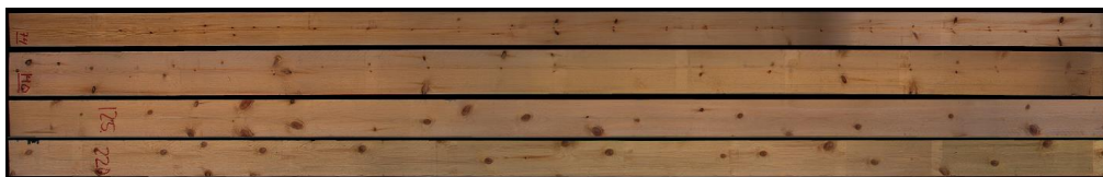
Figure 1. Example of faces of four ID-marked planks, where the two on the top were determined to be sawn from butt logs and the two on the bottom were determined to be sawn from top logs. These images were not used for feature detection by the Boardmaster and were stitched together from three camera images per face after the data collection at the dry-sorting station using a Matlab script.
