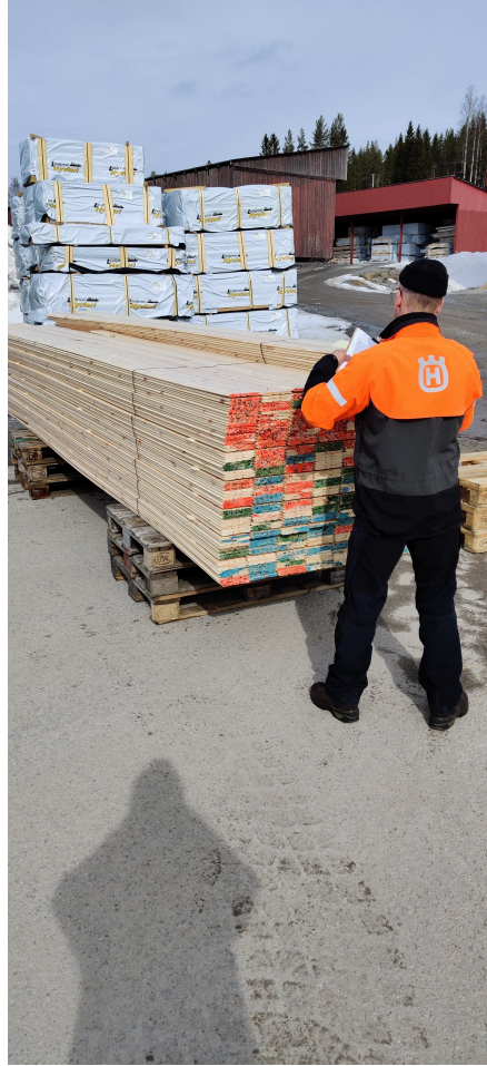
(b) Stacks of wall panels. Each patch of colour is one piece of sawn timber split into a triplet wall panels.
