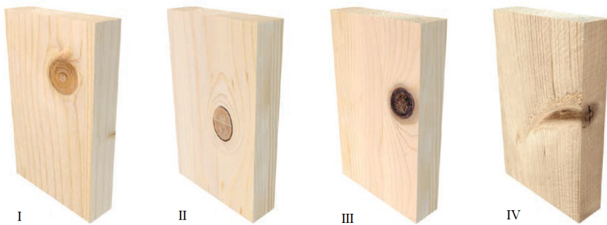
Figure 2.3: Examples of Scots pine knots: I – sound knot, II – dead knot, III – rotten knot, and IV – spike knot, that in this case reaches the edge of the sawn timber. From www.traguiden.se
